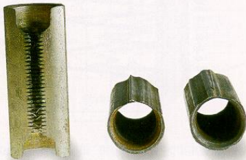
An example of coupling wear as a result of not running rod rotators
