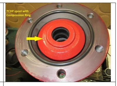
Now you are ready to install the body. Once again, make sure surface flange area top of spool and bottom of Body are clean and free of any debris before mating together.
