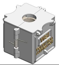
Packing adjustment, (if BSDP is properly maintained), should be achieved by simply turning BSDP cap by hand 1/8" at a time.
