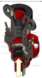
Thread BSDP into pumping tee and tighten until secure connection is achieved between the pumping tee and BSDP.
