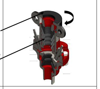
If using a polished rod lubricator, make sure that reservoirs are full of 30W or equivalent oil and **PRESOAK** the wicks prior to starting up pumping unit.
