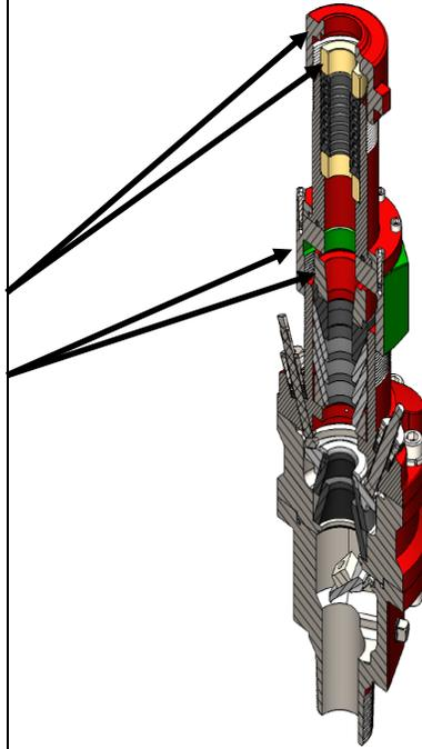
Start unit up and adjust BSPCDP cap only if necessary. You should have a slight film on polished rod as it reciprocates through the BSPCDP. If too much oil is on polished rod, make 1/8" turn adjustments to BSPCDP cap until you have proper film on polished rod.
