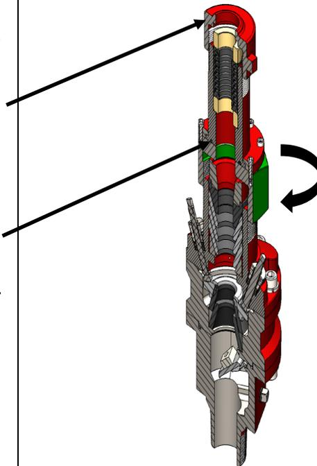
Packing adjustment, if BSPCDP is properly maintained, should be achieved by simply holding BS-ELUG body by hand and turning BSPCDP cap by hand 1/8" at a time.
