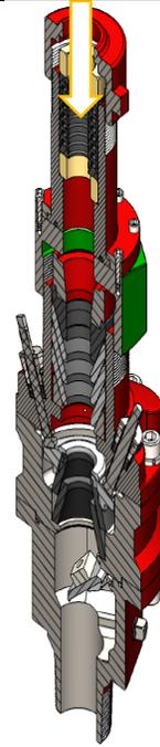
Thread BSPCDP into pumping tee and tighten until there is no leaking between the pumping tee and BSPCDP connection
