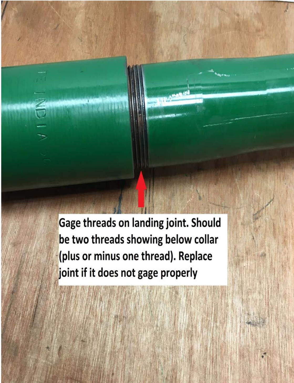
3. If using old tubing or a used sub for the landing, thoroughly clean the threads with a wire brush and dress any MINOR thread damage with a small triangular file or with a thread file. Remove all fittings and gage threads as per step 2.
