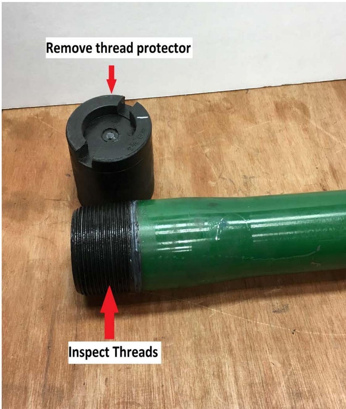
2. In addition to a visual inspection, gauging the threads on the landing joint with a new API monogrammed tubing collar is highly recommended. When collar is installed hand tight, there should be two threads (plus or minus one thread) visible below that collar. Replace the joint if it does not gauge properly.
